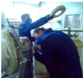
Assembling the NCF reactor in the Weizmann Institute
