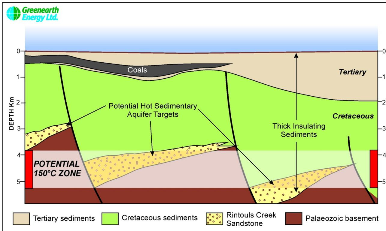
Figure 3. Schematic interpretative cross section showing relationships within the Wombat Geothermal Play.
