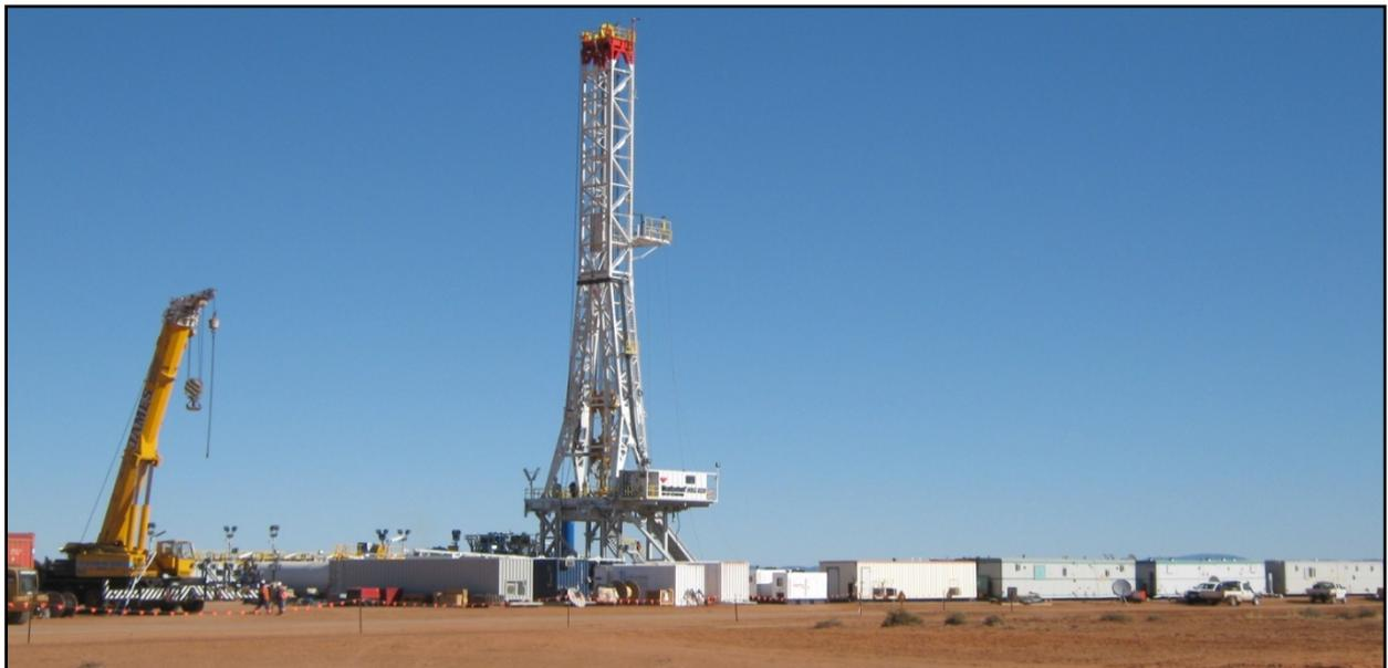
*Figure 1: Weatherford Drilling International Australia Pty Ltd 2,000 HP Drilling Rig 828*
