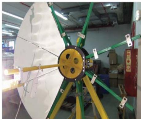
The reflector structure in assembly
